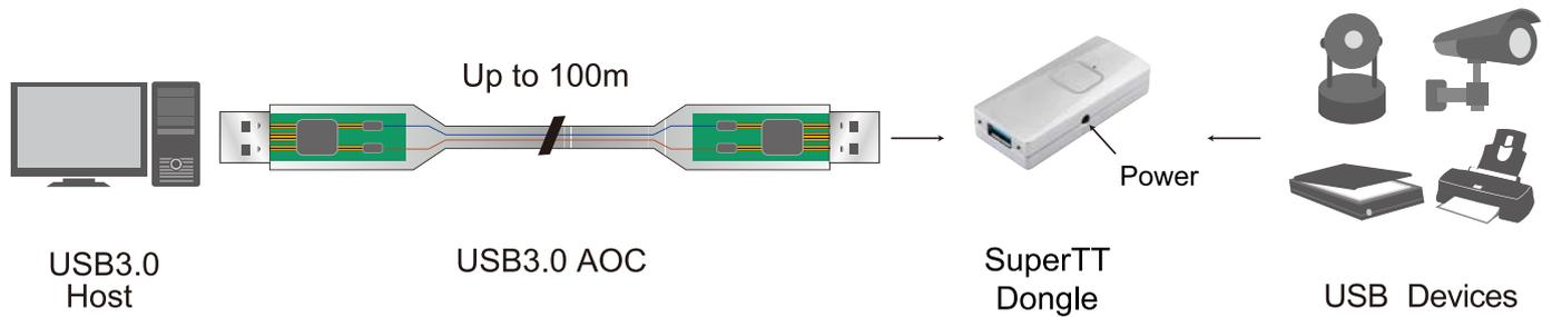
\*USB 3.0 Active Optical Cable is only backward compatible with USB 2.0 when connected with SuperTT Dongle
